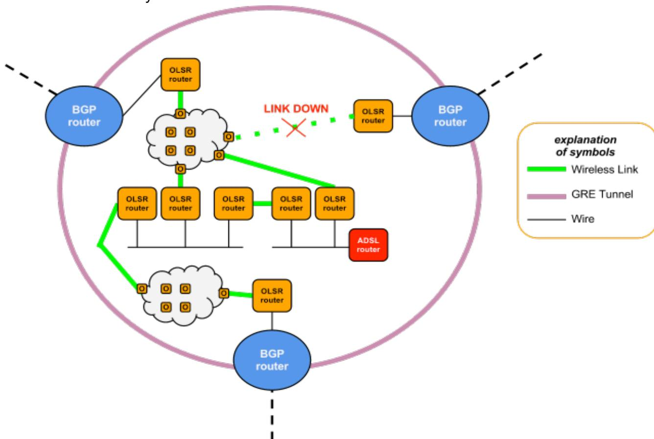
As we see in the figure, we want to handle the scenario in which the BGP router loses its connectivity to its OLSR 2-hop neighbor because the wireless link is down. In this case we need the BGP router to stop announcing upstream the public IPv4 and IPv6 routes of Ninux.
