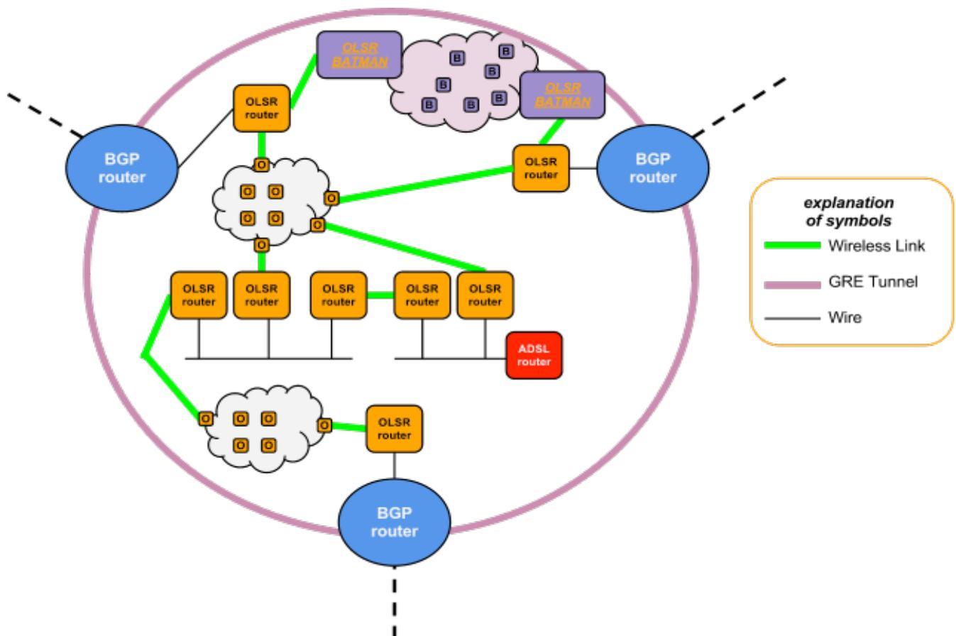
For what concerns the batman-adv nodes, as for the stub area, they do not have any knowledge about the L3 routing issue, therefore they will continue to use as default gateway the edge router assigned by the DHCP protocol.
