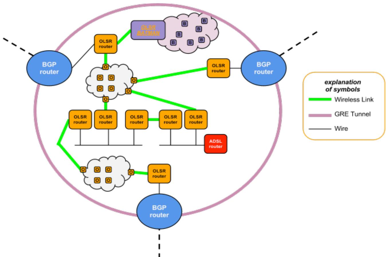
As we see in the figure there will be an edge OLSR router between the two domains that speaks both the OLSR and the B.A.T.M.A.N.-Advanced routing protocol. This edge router will announce all the IP addresses used in the batman-adv network with an HNA setting.
